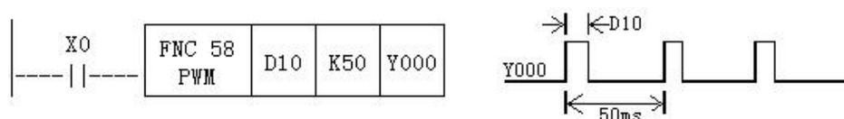
In this example, the data range of D10 is changed from 0 to 50, and the average output of Y0 is 0 to 100%. If D10 data >50, it will be wrong.
