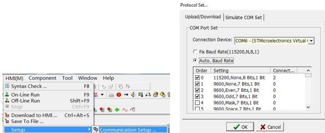
Specify the communication port of the PC in the [Upload/Download] of the communication setting window, that is, the port where the download cable is connected to the PC. For example, COM24, you can select [Use fixed communication rate] in conjunction with HMI [download screen], or let the PC automatically try to download at different rates.
