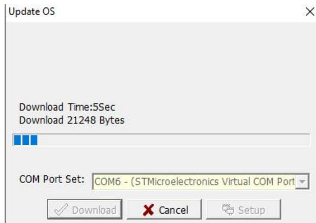
Step 4: After the download is complete, restart the power of the HMI.
