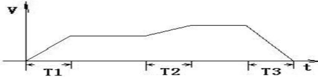
Acceleration and deceleration time T calculation: (target speed - current speed) \* Acceleration and deceleration time/maximum speed
