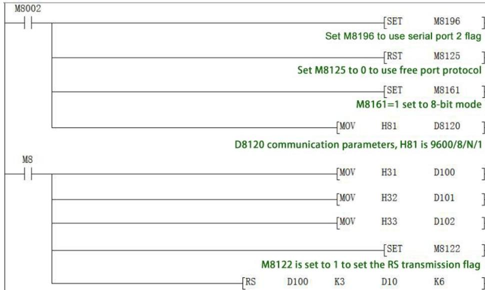
Use the serial port tool by serial port 2 to monitor the data obtained is
