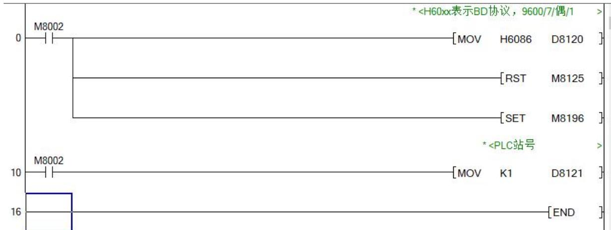
The touch screen sets the BD protocol master station, that is, it can communicate with the PLC.
